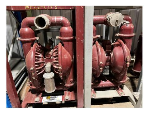
Diaphragm type pumps are an air operated, positive displacement, self-priming pump designed for demanding applications that require a robust design.
