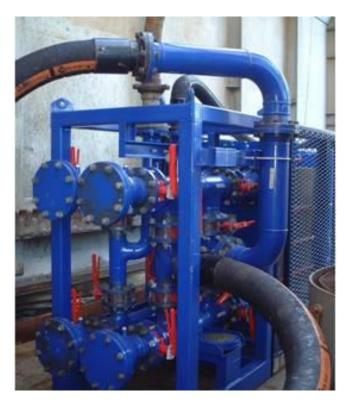
The cooling system, featuring Alfa Laval plate-type heat exchanger for cooling the drilling fluid for high pressure/high temperature wells, for increased safety. The unit is very compact, and skid mounted, consists of either a single or dual plate heat exchanger depending on process requirements designed in accordance to ASME codes and standards.
