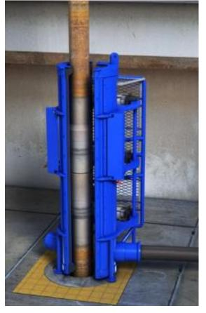
The mud bucket clamps around the pin and box ends of the drill pipe creating an airtight seal.
