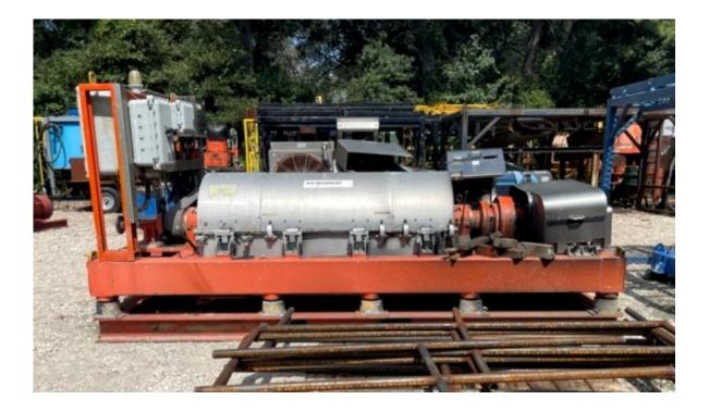
High volume design for very low gravity solids (LGS) and barite recovery.)
