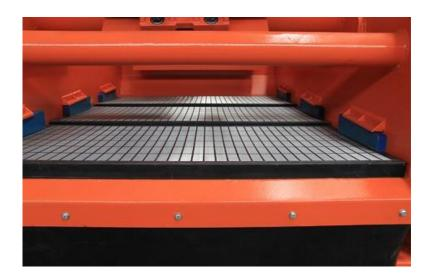
Composite Screens provide higher surface tension. When using powder-coat, the applied temperature is lower than when the product is moulded.
